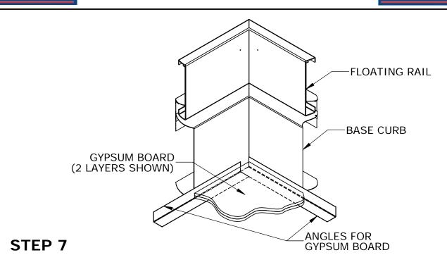
If required, install field supplied gypsum board in location specified on submittal. Place on Cambridgeport supplied angles on interior of isolation curb.
