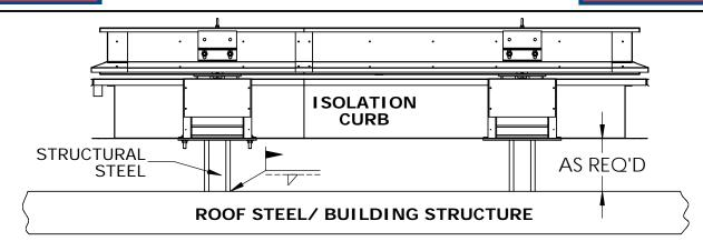
If site conditions require an increase to the installed height of the curb, wood blocking is not an acceptable method. Structural steel must be used to adequately transfer and resist any wind and/or seismically induced loads on the equipment. Please consult factory for additional details and requirements.
